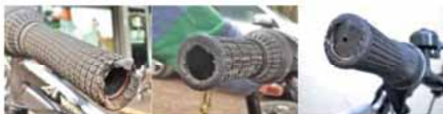
Figure 1: Exposed metal handlebar ends
